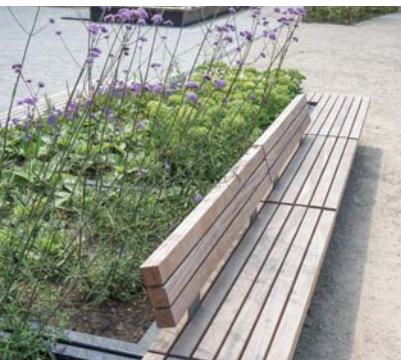
RAISED POWDER COATED ALUMINIUM PLANTER EDGE WITH INTEGRATED SEATING EDGE
