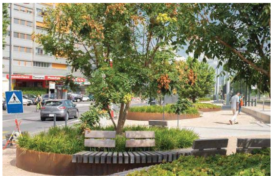
RAISED POWDER COATED ALUMINIUM PLANTER EDGE WITH INTEGRATED SEATING EDGE
